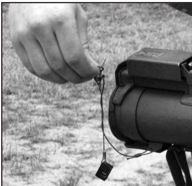
Figure 3-49. Removing the M72A2/A3 transport safety pin.
