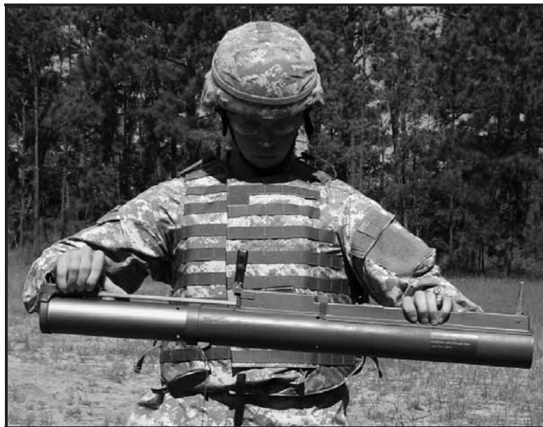
Figure 3-51. Extending the M72A2/A3 launcher.
