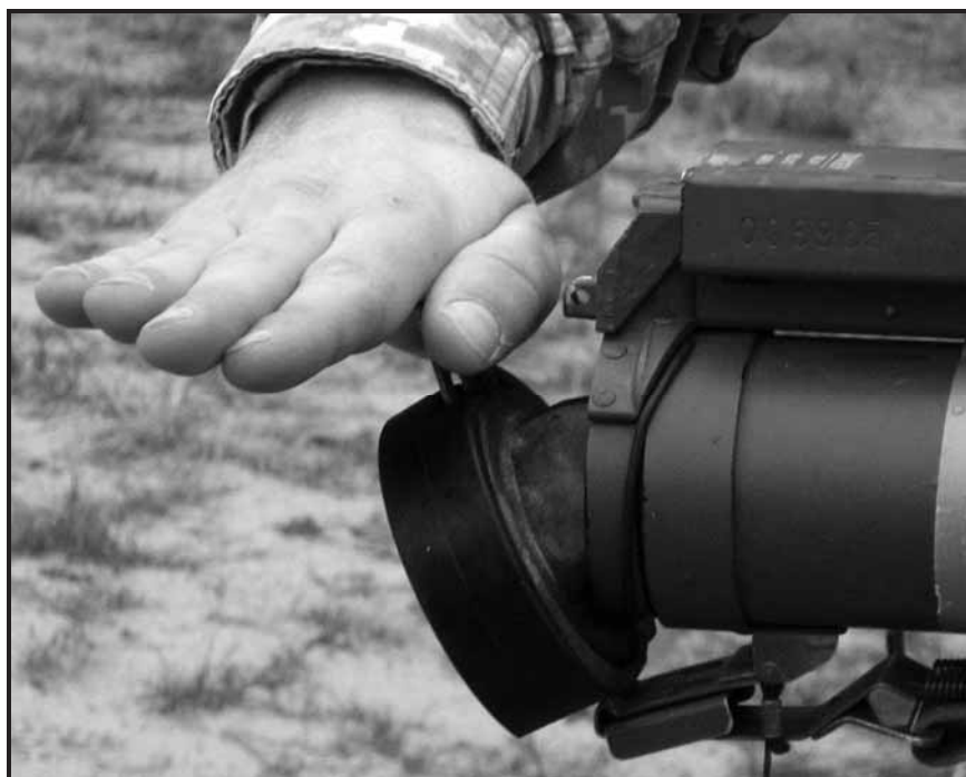
Figure 3-44. Releasing the improved M72 rear cover/shoulder stop.
