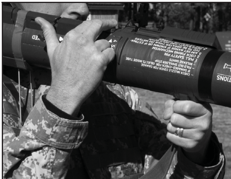
Figure 3-29. Releasing the red safety release catch on the M136 AT4.
