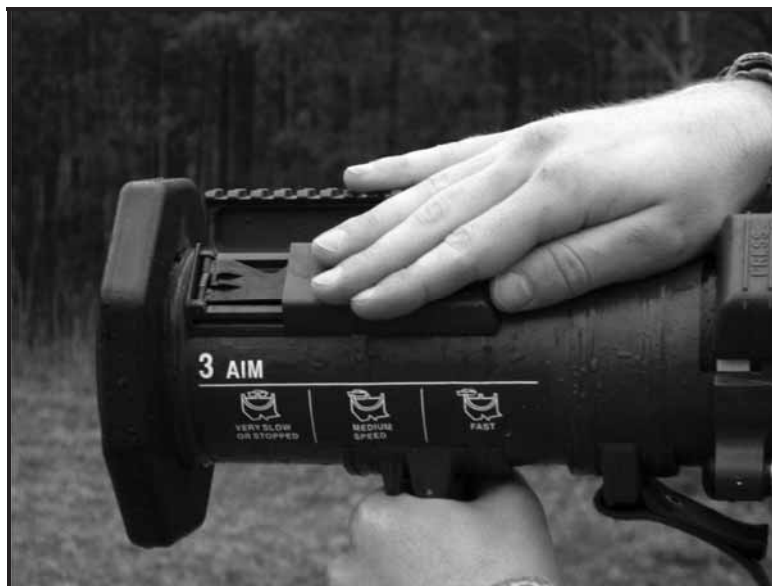
Figure 3-36. Opening the front sight cover on the M136A1 AT4 confined space.
