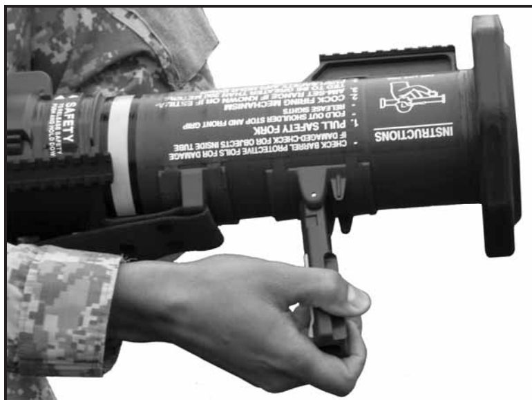
Figure 3-34. Unfolding the front grip on the M136A1 AT4 confined space.
