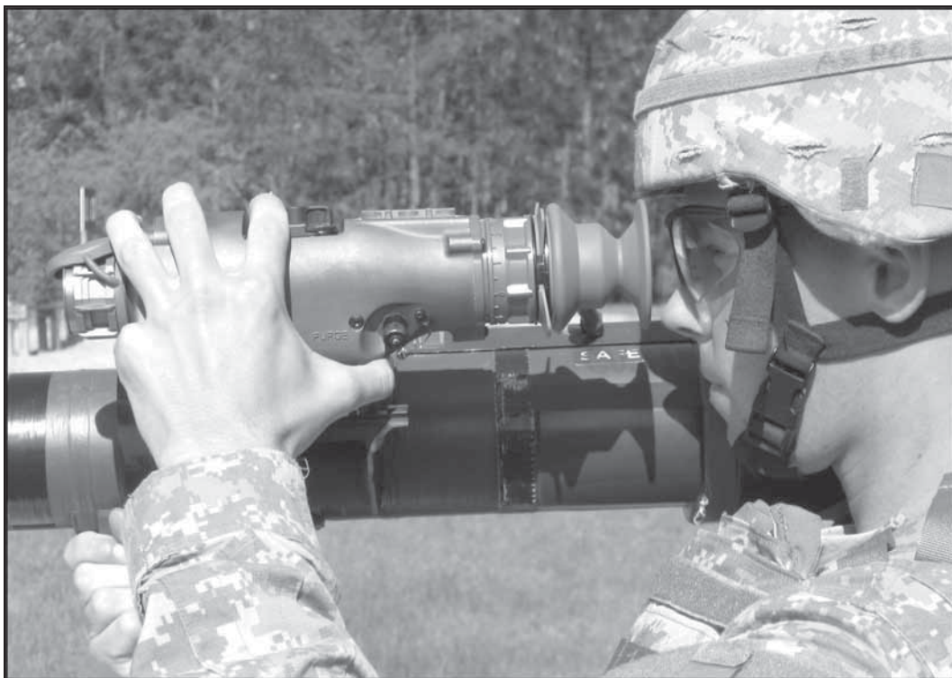
Figure C-11. Finding night vision sight eye relief on the M136 AT4.
