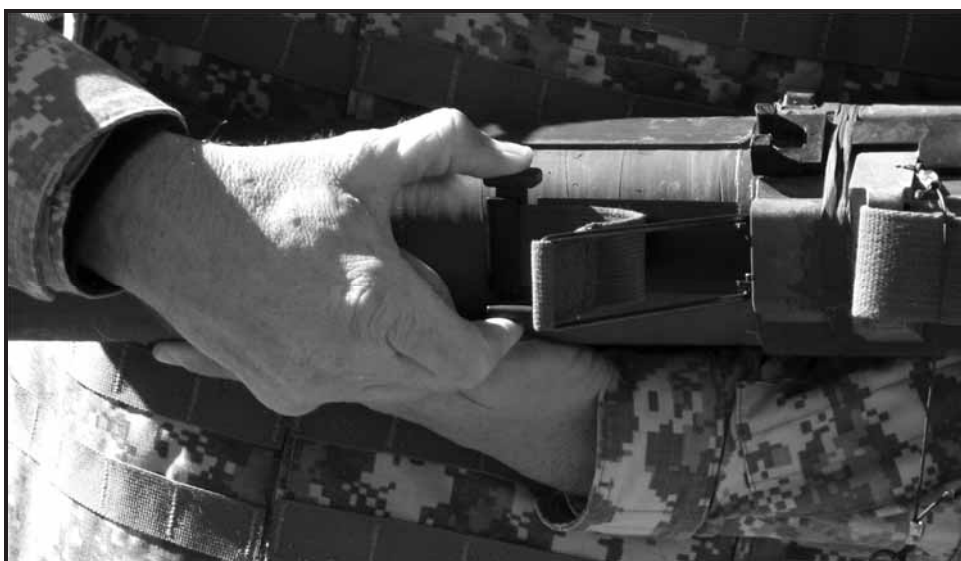
Figure 3-18. Unlocking and unfolding the shoulder stop on the M141 bunker defeat munition.
