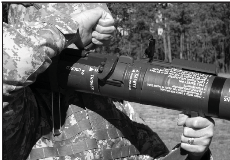
Figure 3-27. Cocking the M136 AT4.
