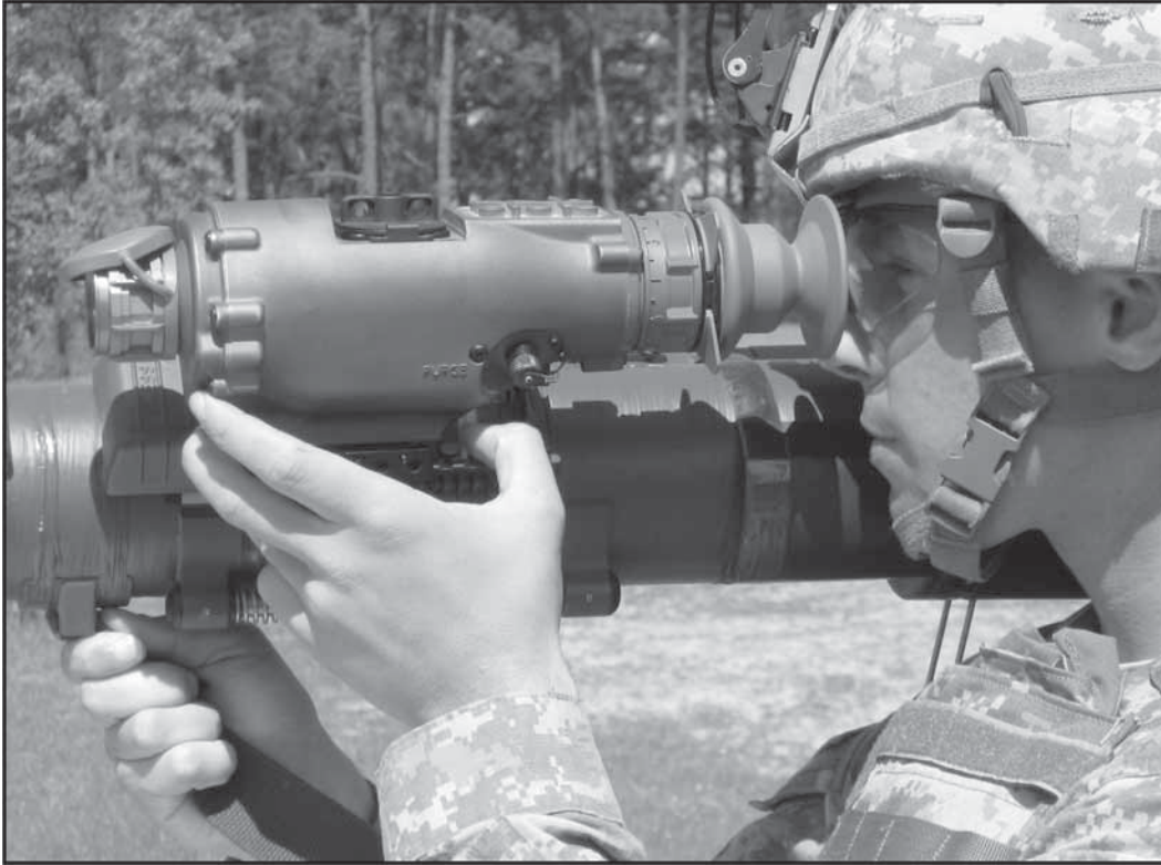
Figure C-13. Finding night vision sight eye relief on the M136A1 AT4 confined space.
