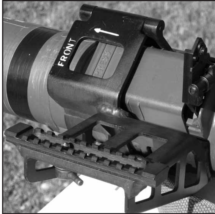
Figure C-10. M136 AT4 with night vision device mounting bracket attached.
