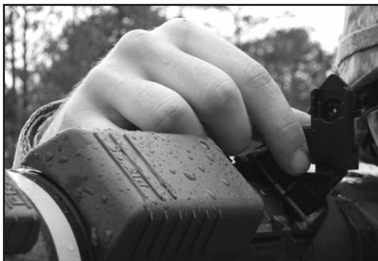
Figure 3-28. Adjusting the rear sight on the M136 AT4.
