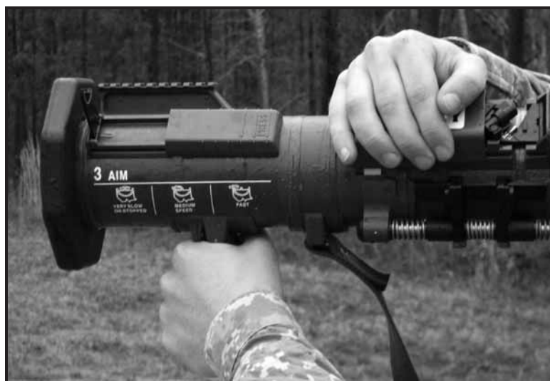
Figure 3-37. Opening and adjusting the sights on the M136A1 AT4 confined space.
