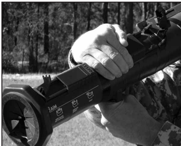
Figure 3-26. Opening the sights on the M136 AT4.
