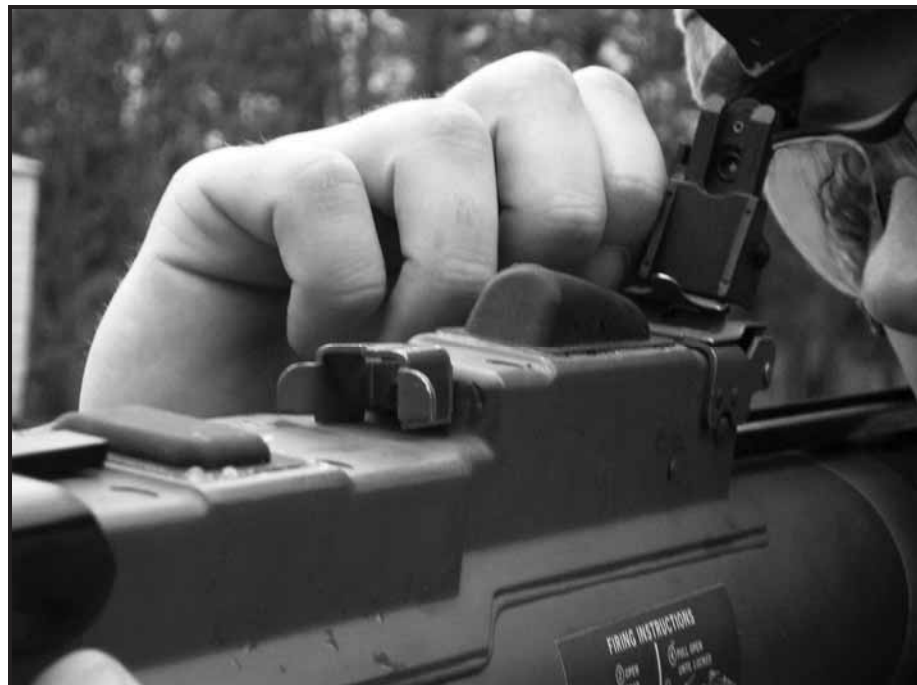
Figure 3-46. Adjusting the rear sight on the improved M72.
