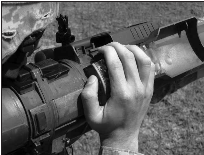
Figure 4-12. Trigger manipulation of a M141 bunker defeat munition.
