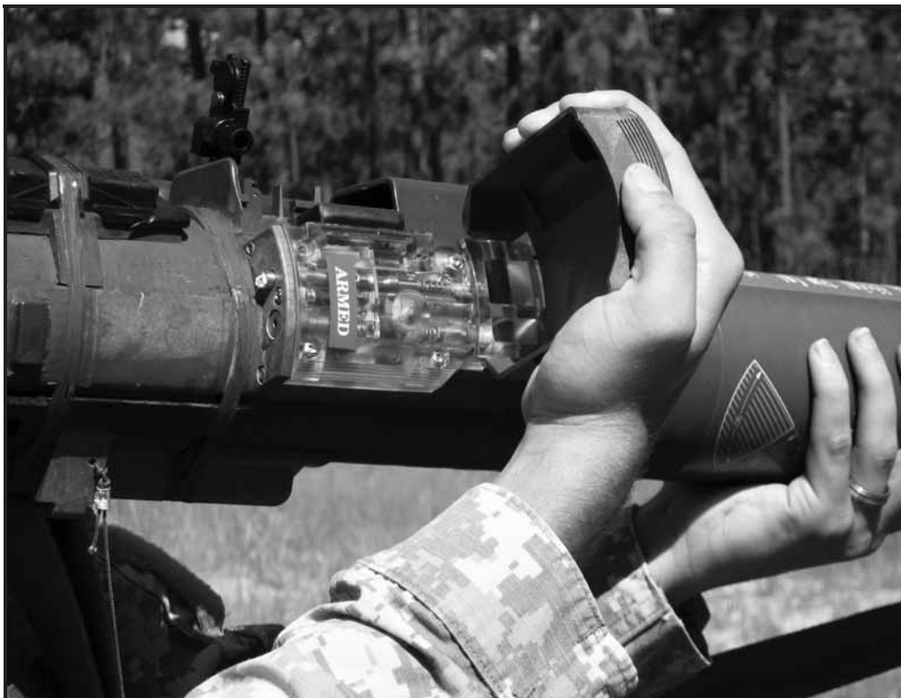
Figure 3-20. Arming the firing mechanism on the M141 bunker defeat munition.
