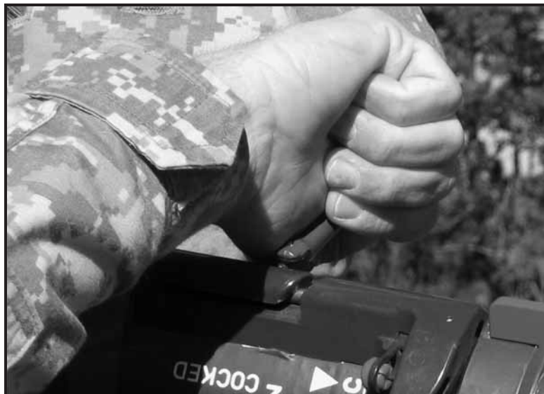
Figure 3-38. Cocking the M136A1 AT4 confined space.
