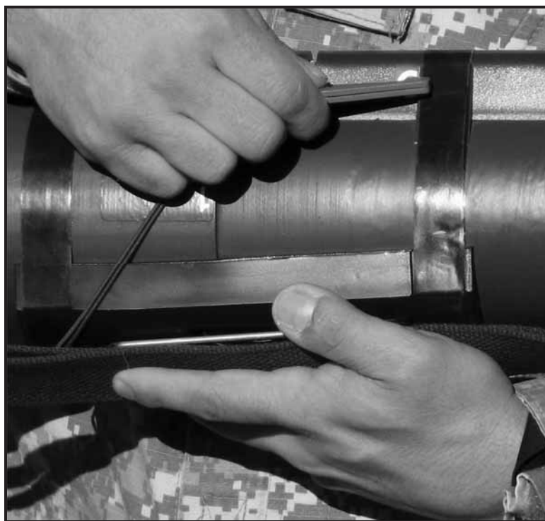
Figure 3-32. Removing the transport safety fork on the M136A1 AT4 confined space.
