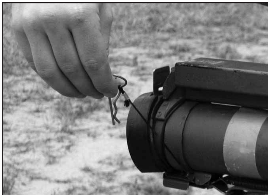
Figure 3-43. Removing the improved M72 transport safety pin.
