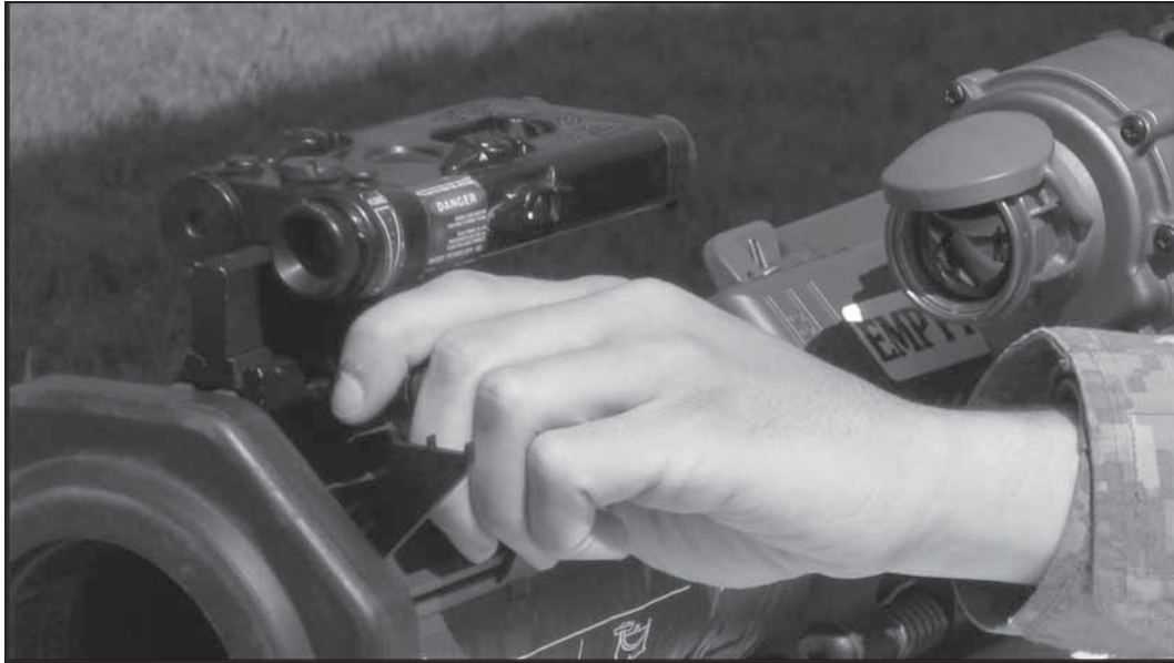
Figure C-14. Securing the laser aiming light/illuminator to the M136A1 AT4 confined space.
