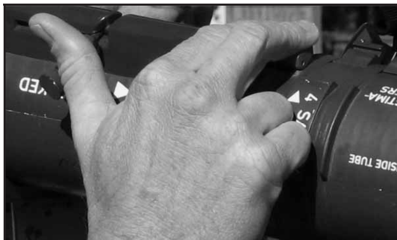
Figure 3-40. Releasing the red safety catch on the M136A1 AT4 confined space.
