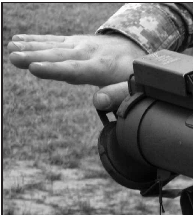
Figure 3-50. Removing the M72A2/A3 front cover and the adjustable sling assembly.
