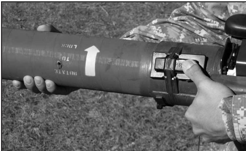
Figure 3-17. Locking the M141 bunker defeat munition inner tube.
