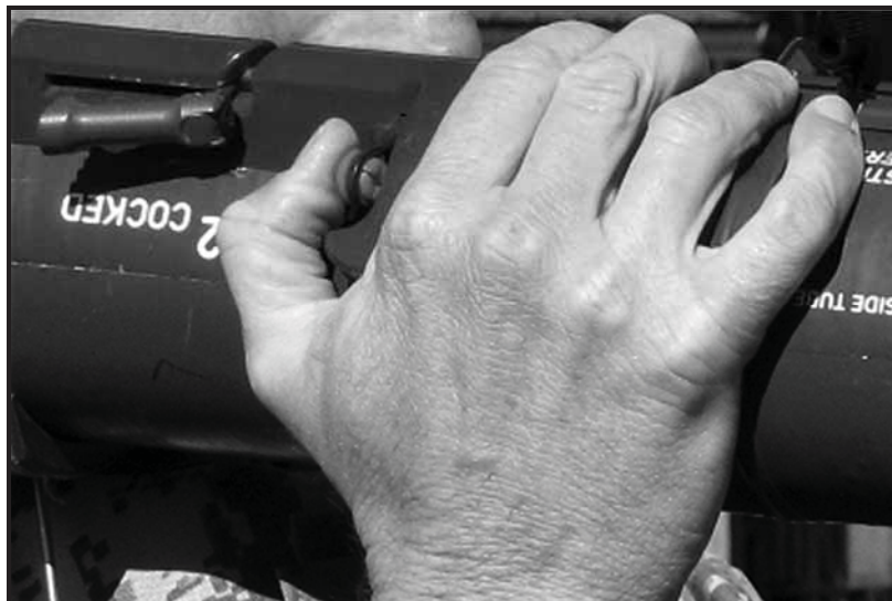
Figure 4-13. Trigger manipulation of a M136-series shoulder-launched munition.
