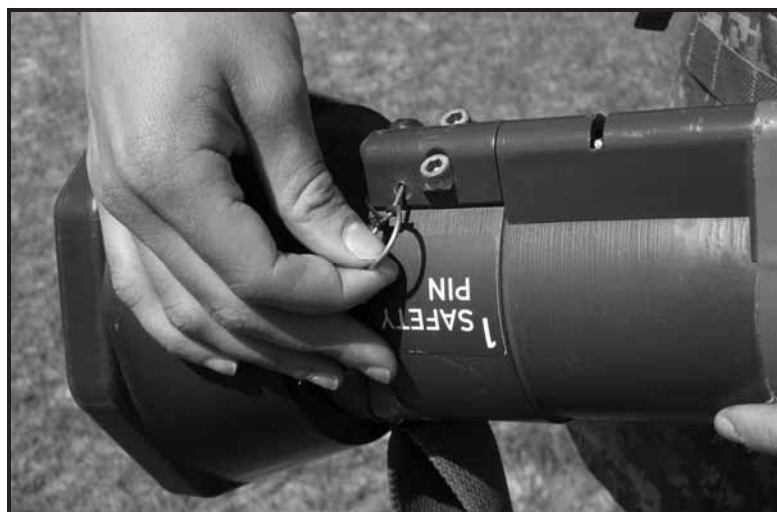
Figure 3-24. Removing the transport safety pin on the M136 AT4.
