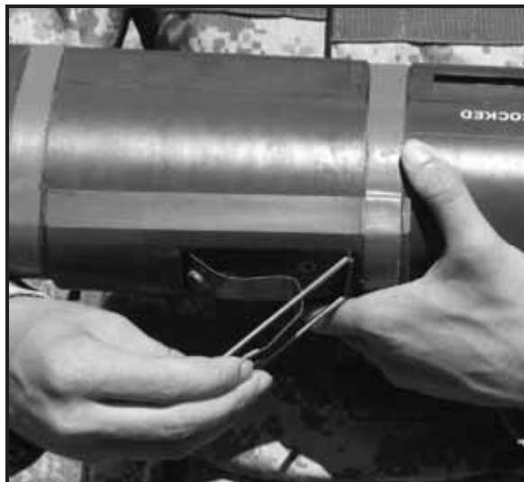
Figure 3-25. Unsnapping the shoulder stop on the M136 AT4.
