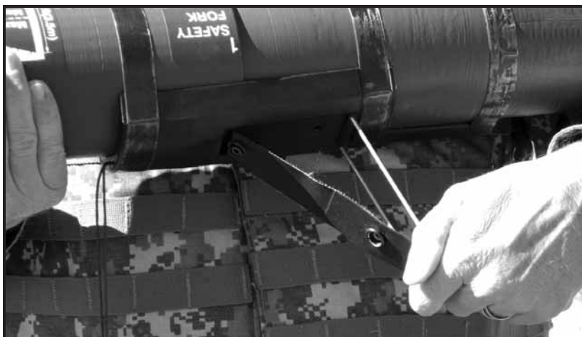
Figure 3-33. Unsnapping the shoulder stop on the M136A1 AT4 confined space.
